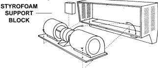
Figure 4 - Removing Motor/Blower Assembly
